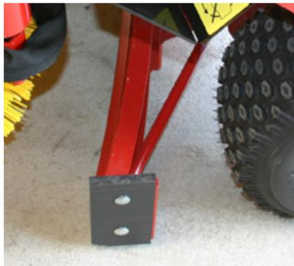
Rubber on scraper can be replaced.
