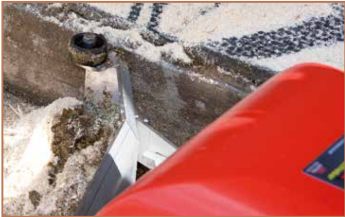
Side run-up rollers mounted on the scraper
