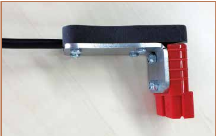
Charging plug with strain relief and handle
