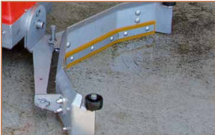
Cleaning strip made of polyurethan (reversible)
