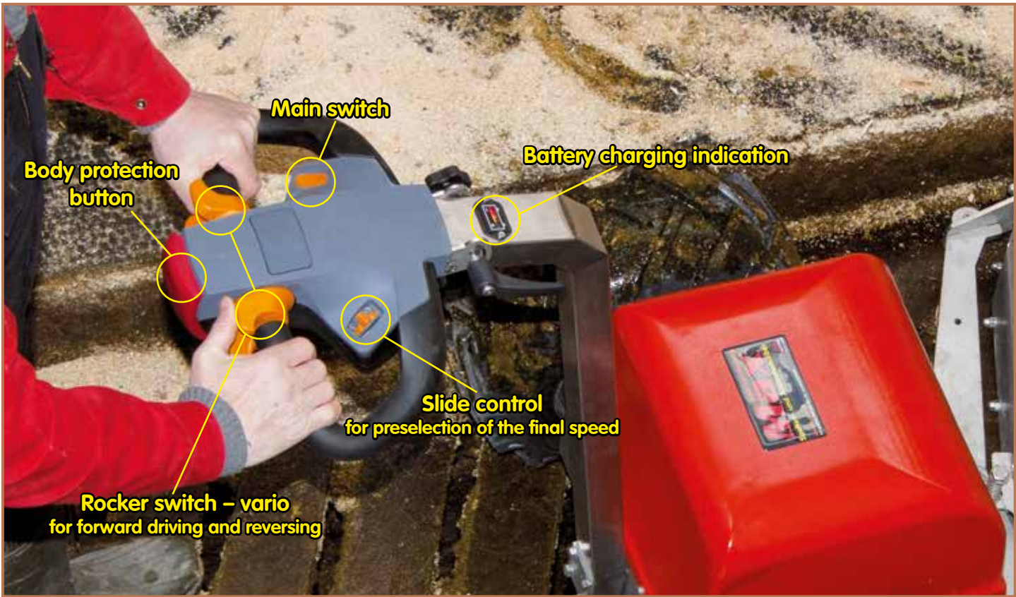
Ergonomically shaped tiller head for relaxed operation
